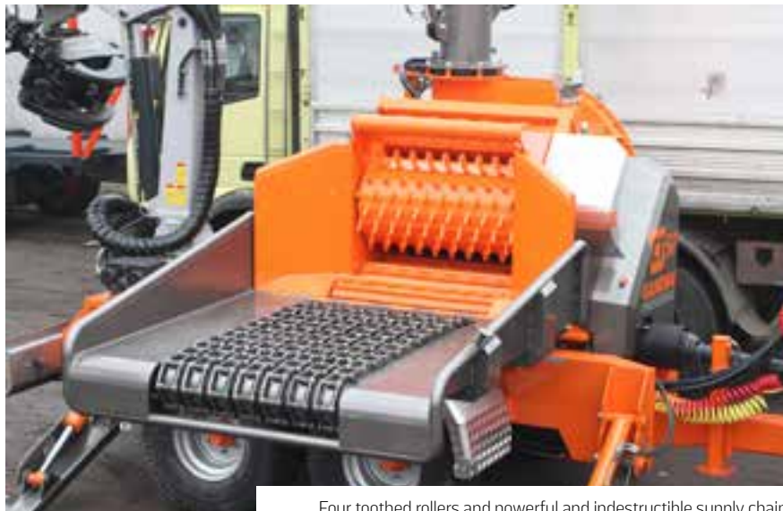
Four toothed rollers and powerful and indestructible supply chain
