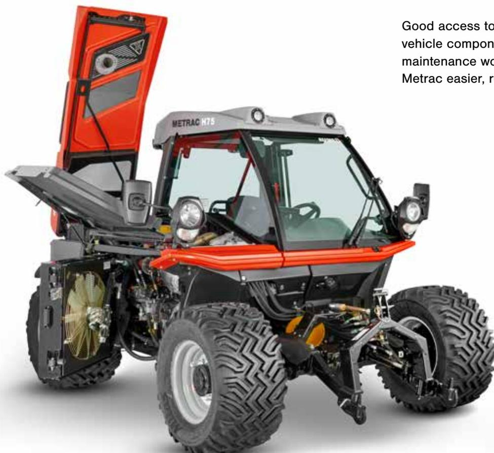
Good access to the most important vehicle components makes maintenance work on the new Metrac easier, reducing downtime.
