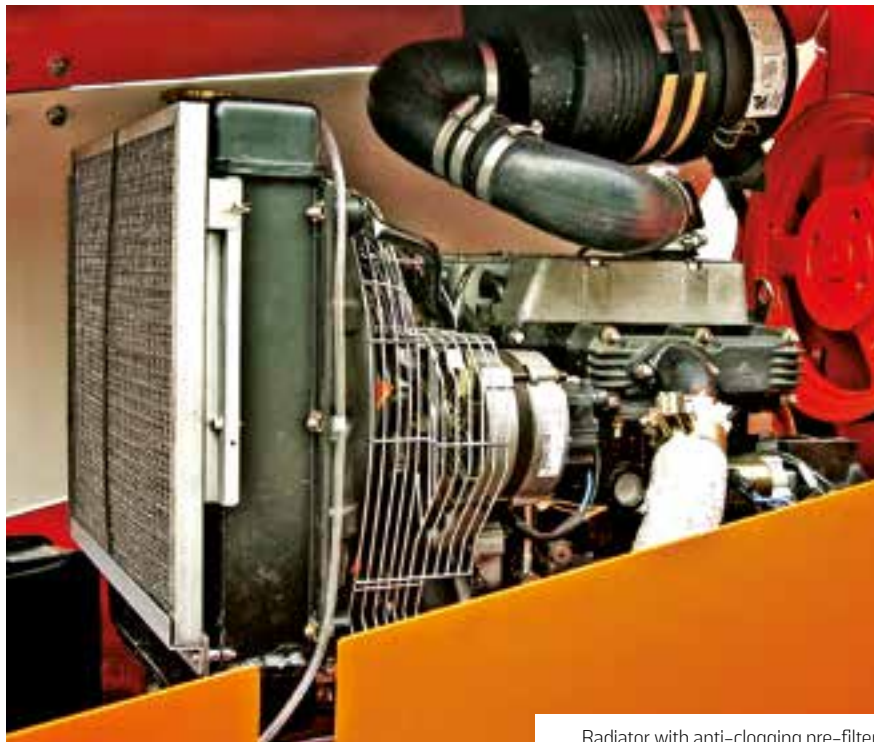
Radiator with anti-clogging pre-filter
