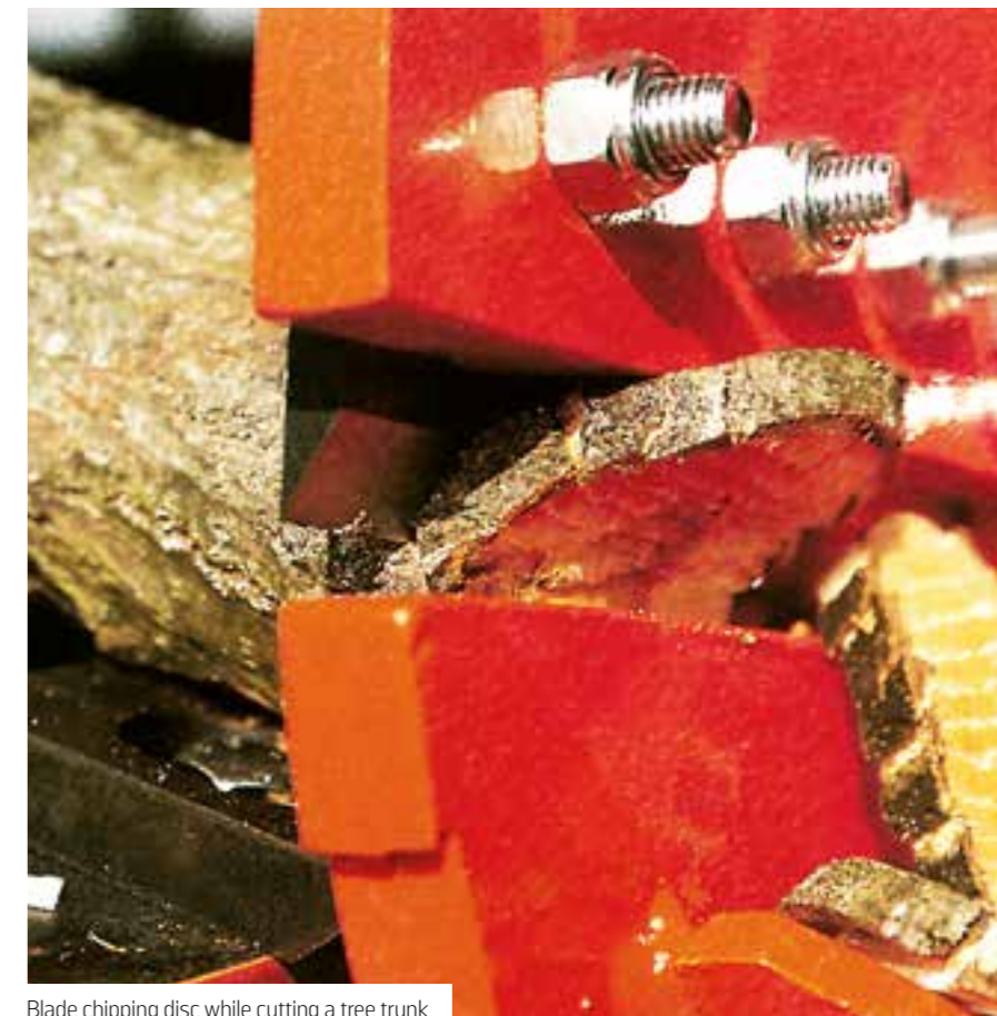
Blade chipping disc while cutting a tree trunk
