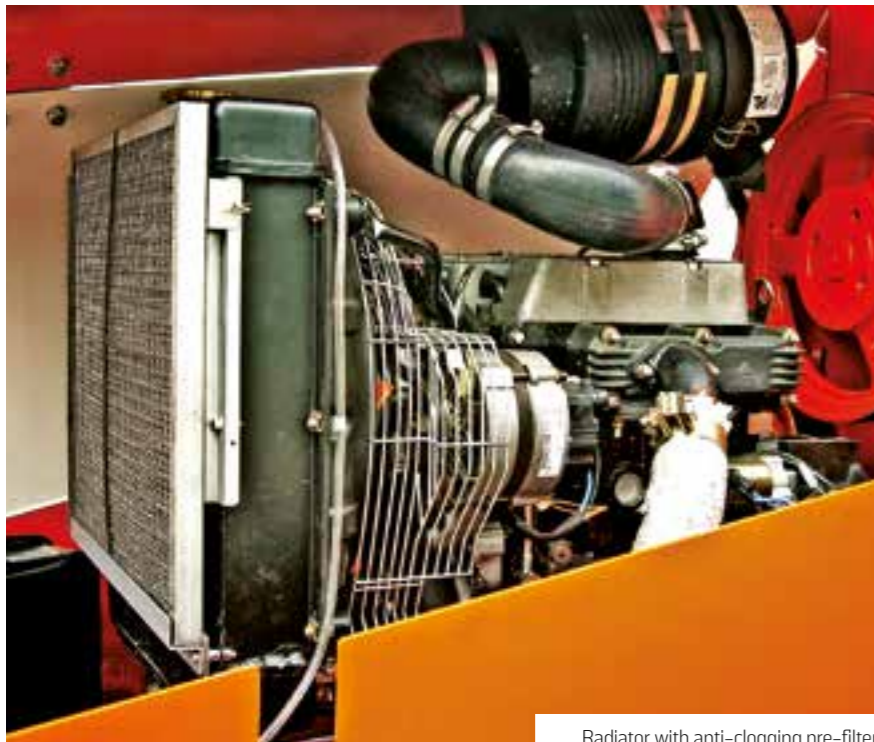
Radiator with anti-clogging pre-filter
